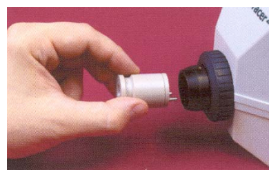
The pre-concentrator dramatically boosts sampling efficiency
